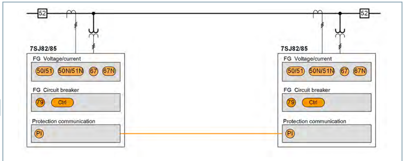
Figure 2.3/3 Fast Fault Clearing in Lines with Infeed at 2 Ends
