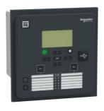
universal protection relay, PowerLogic P3U30, 4L ringlug, 4U, 16DI/8DO, Uaux: 48-230V, DI: 110-230V, 2 x RJ-45
