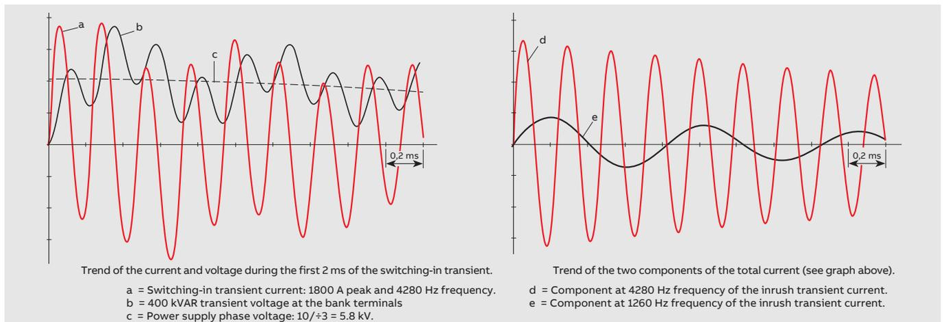
Fig.G: Example of a current transient when a capacitor bank is switched-in with another already supplied.
