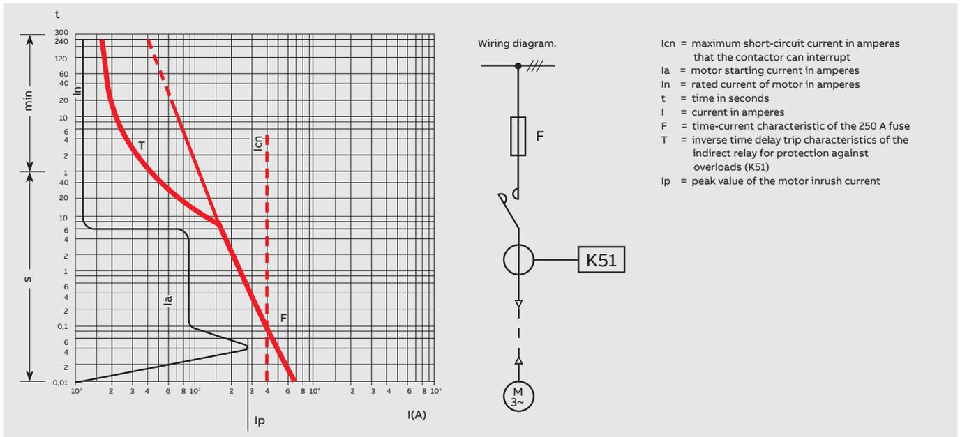
Fig. E - Graph showing coordination between the 250 A ABB CMF fuse and inverse time delay trip release.
