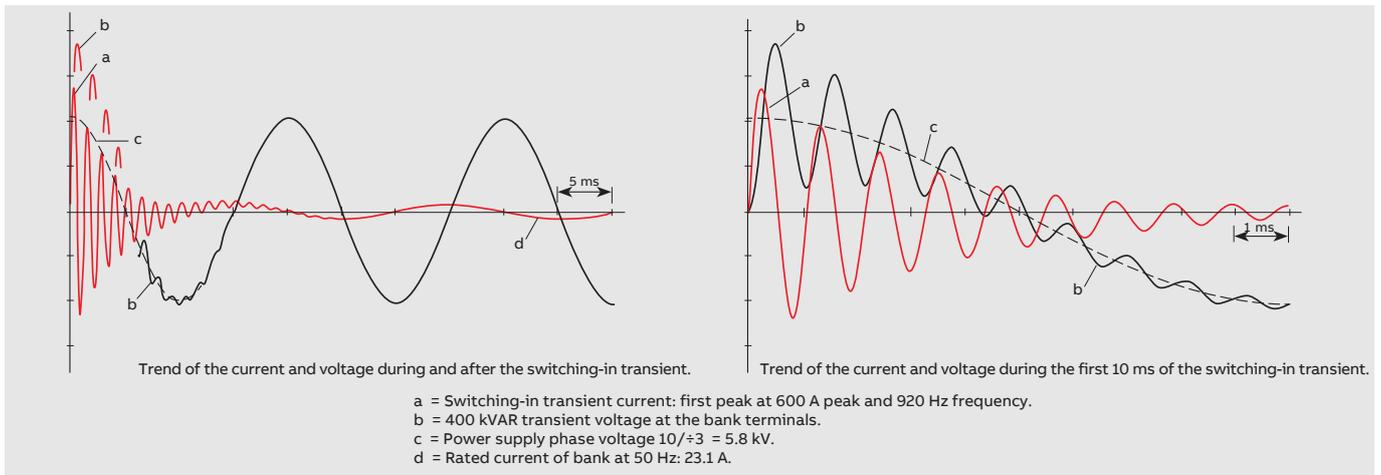
Fig. F: Example of a current transient when a single capacitor bank is switched-in.
