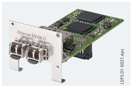
Fig. 11/49 Optical Ethernet communication module for IEC 61850 with integrated Ethernet switch
