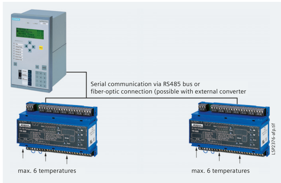
Fig. 8/9 Temperature measurement and monitoring with external thermo-boxes
